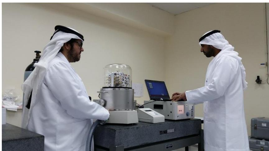
Figure 2. The 7 MPa gas pressure standard at EMI
