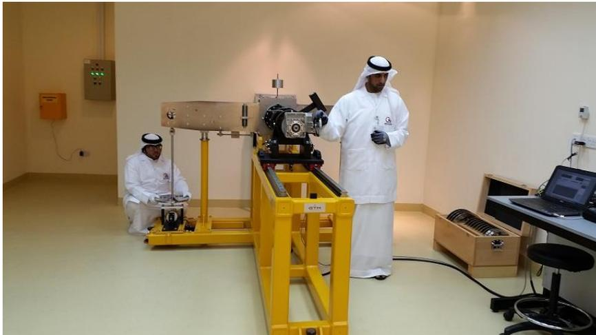
Figure 1. The 1000 N·m torque standard machine at EMI
